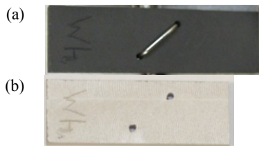
Fig. 4. (a) Typical graphite coupon appearance prior to exposure to FLiNaK at 850C for 1000 hours. (b) Graphite coupon after cleaning showing the presence of the chrome carbide coating. Sample is shorter because a cross section of the sample had been taken prior to photographing.
