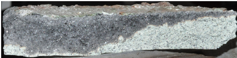
Fig. 3. Cross section of the clay bonded SiC base plate used in the high temperature furnace. Affected areas are discolored black with some associated swelling.
