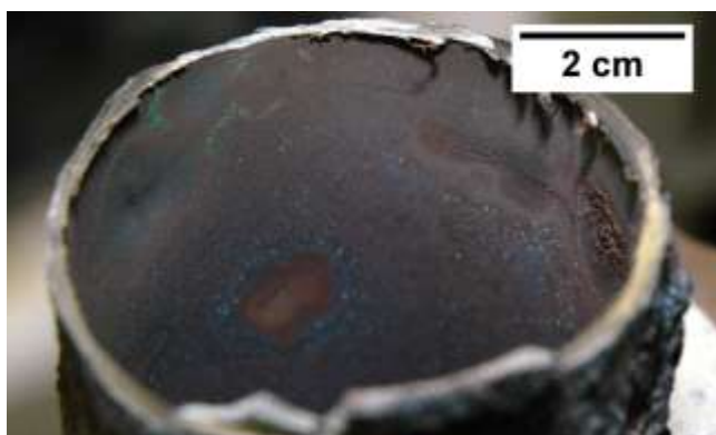
Figure 55. Circumferentially aligned stress cracking on the interior of one of the static test crucibles.
