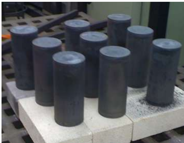
Figure 10. Crucibles from test 1 following removal from the furnace after 1000 hours.
