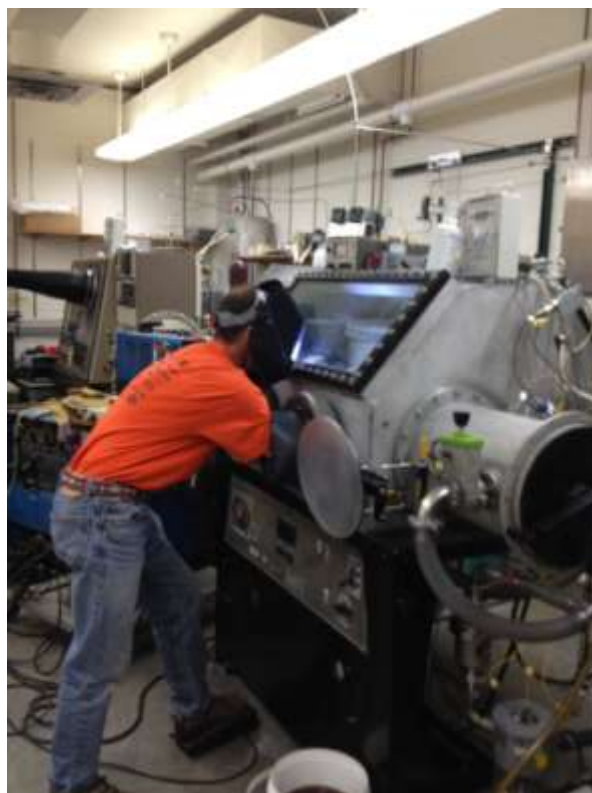
Figure 13. Crucibles being welded in argon atmosphere glove box.
