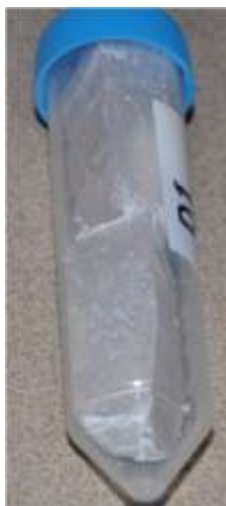
Figure 8. Metallic sodium used in the static corrosion tests.
