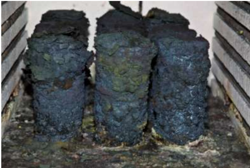
Figure 52. Photograph of crucibles at the conclusion of the 1000 hour static test.
