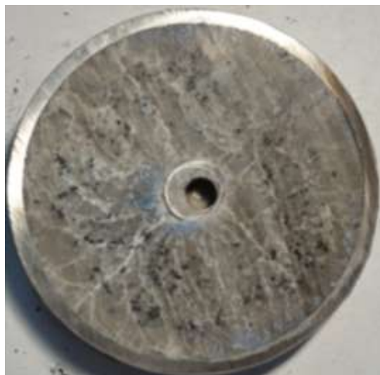
Figure 49. Graphite particle dispersion within frozen FLiNaK in a crucible containing 316L, graphite and metallic sodium held for 1000 hours at 850°C.
