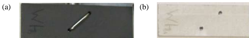
Figure 46. (a) Typical graphite coupon appearance prior to exposure to FLiNaK at 850°C for 1000 hours. (b) Graphite coupon after cleaning showing the presence of the chrome carbide coating. The length is shorter because a cross section of the sample has been taken.
