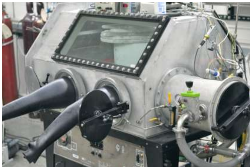
Figure 3. Argon glove box facilities at the University of Wisconsin-Madison.
